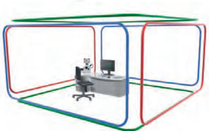
Bilz magnetic field compensation using room coils
